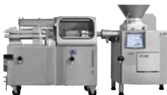
↑ PVLH 241 with GD 93-3 inline grinding system
