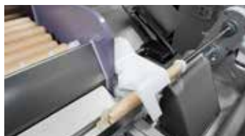
↑ Sausage casing magazine with automatic slug casing spooling
