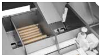
↑ Sausage casing magazine and spooling rail for automatic casing spooling
