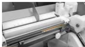
↑ Sausage casing magazine and spooling rail for automatic casing spooling
