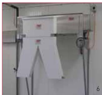
RVH on wall console with Y chute for two ice outlets
